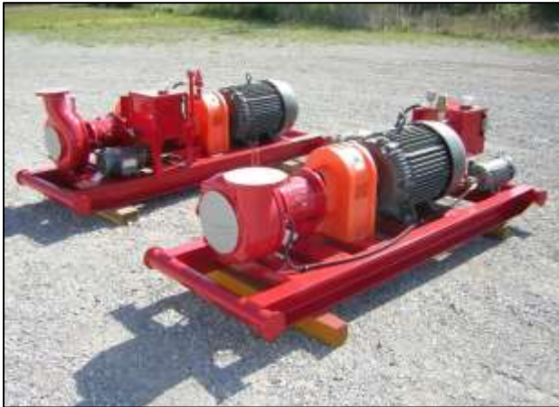
Cementing Pump w/ Speed Increasers and Lip Seal Lubrication System
